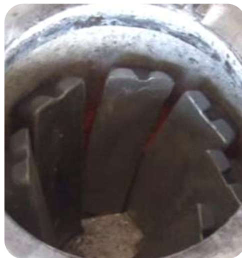
Loosely charged ingots
