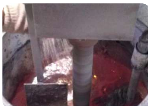
Adding Granular Flux
