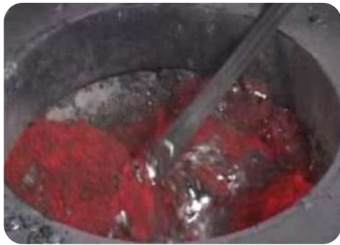
Stirring Oxide and Dross
