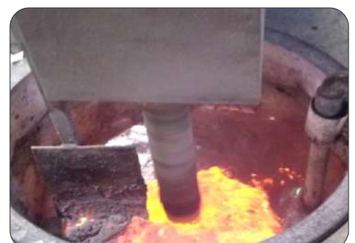
Churning, Cleaning, Degassing
