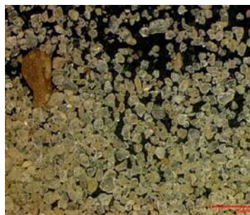
Indian Sand shape under microscope
