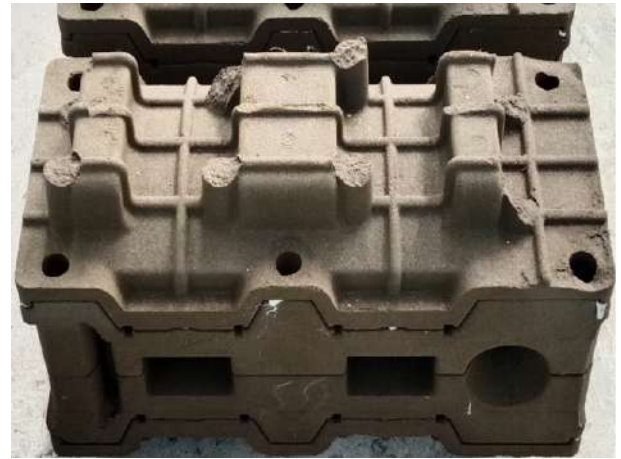
Fig. 3 – Shoted mould with ribs
