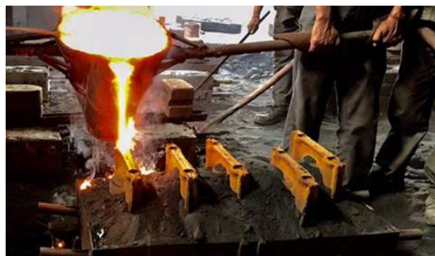
Figure 1 - Dump Box Mould Pouring with sand backing.
