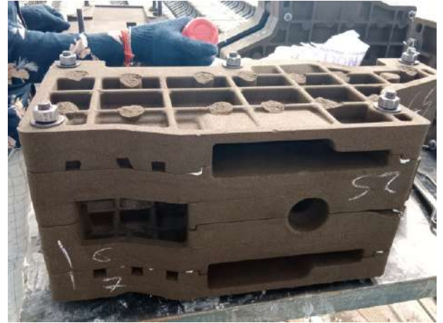
Fig. 5 – Clamped mould - ready to pour.
