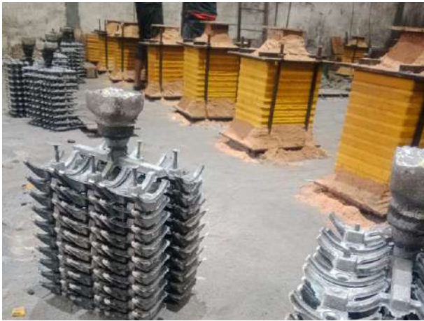
Fig. 4 – Double side shoted stack Mould
