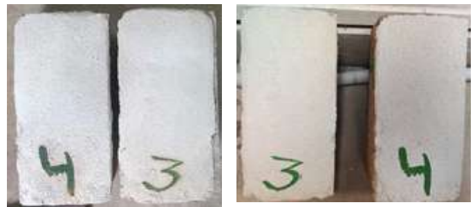
Fig.3: Appearance of water based neutral ramming mass (Left – after firing at 1600°C, Right – after firing at 1000°C) suitable for patching purpose
