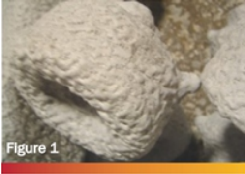
Photos from left to right show parts experiencing cracking. Positive metal and permeability defects.
