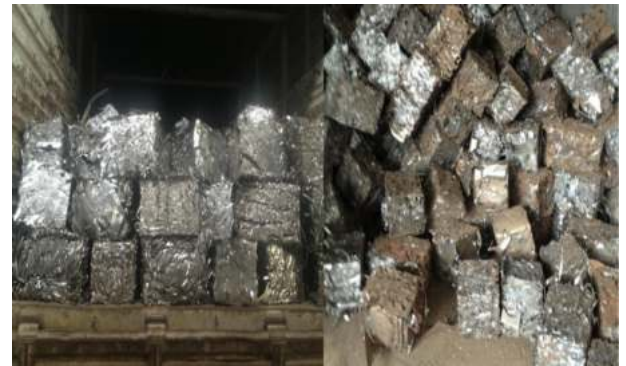
Fig 3: Compacted CRC Scrap
