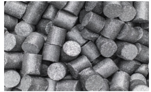
Fig 5: Briquetted metal borings /Chips
