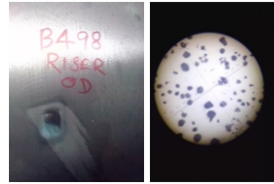
In Fig.2 Test result shows the following specification requirement 90% Form VI nodularity according to ISO945.
